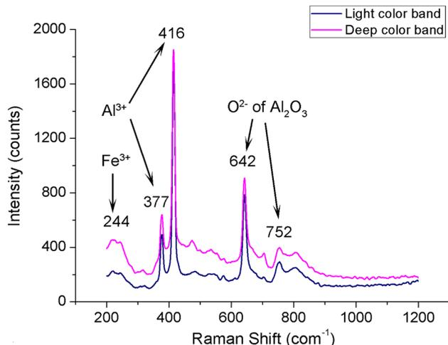
Fig. 5. Raman spectrum of SC2.
