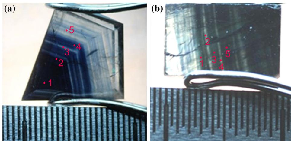
Fig. 2. Dotting position of samples by LA-ICP-MS: (a) dotting sequence of sample SC1 and (b) dotting sequence of sample SC2.
