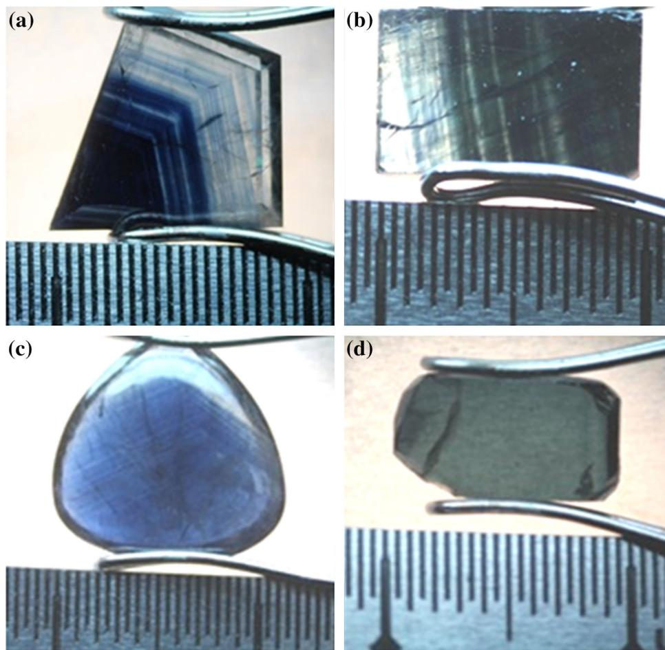
Fig. 1. Sample photos, the calibration of scale is 0.5 mm: (a) sample SC1 (b) sample SC2, (c) sample SC3, and (d) sample SC4. The sample photos were taken in the dark-field lighting condition of gem microscope.
